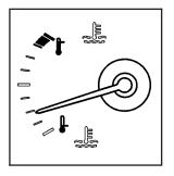
This gage shows the engine coolant temperature.
